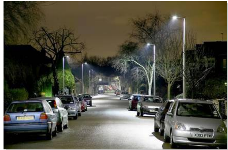
Ceramic Discharge Metal Halide (CDMH) - CRI 65-75
